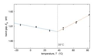
Fig. 5 Band gap (eV) (black dots) for perovskite composition  $Cs_{0.17}FA_{0.83}Pb(Br_{0.17}I_{0.83})_3$  as a function of temperature (°C), calculated from up and downward cycles of EQE, with a linear fit before discontinuity (blue dashed line) and after slope discontinuity (red dotted line). The grey dashed line shows the intersection of the two fit slopes.
