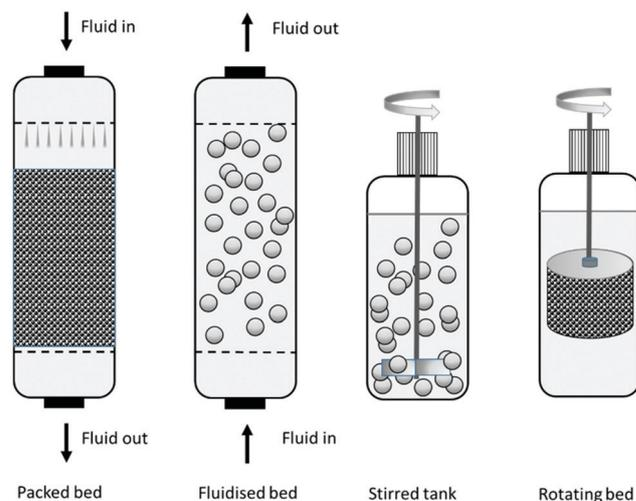
Fig. 8 Reactor design.
