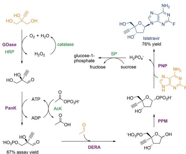
**Scheme 9** *De novo* enzymatic synthesis of islatravir. GOase: galactose oxidase; PanK: pantothenate kinase; DERA: deoxyribose 5-phosphate aldolase; PPM: phosphopentomutase; PNP: purine nucleoside phosphorylase; HRP: horseradish peroxidase; Ack: acetate kinase; SP: sucrose phosphorylase. Starting materials are highlighted in orange. The product is highlighted in blue. Key enzymes in synthetic routes are highlighted in purple. Auxiliary enzymes are highlighted in green.
