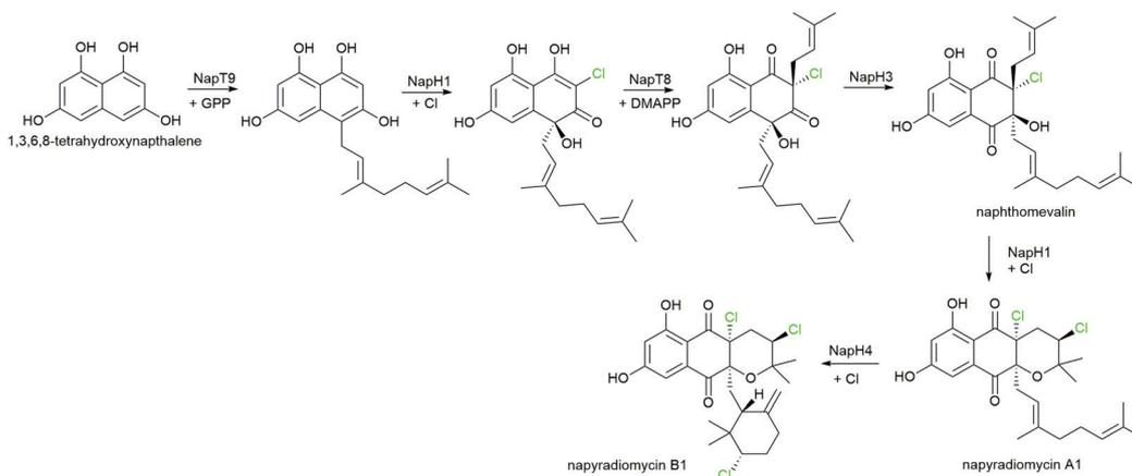
**Scheme 7** Novel enzymes, enzymatic mechanisms and cascades for the synthesis of Napyradiomycins. GPP: geranyl diphosphate; DMAPP: dimethylallyl diphosphate; NapH1, H3, and H9: vanadium-dependent haloperoxidases; NapT8 and T9: aromatic prenyltransferases.
