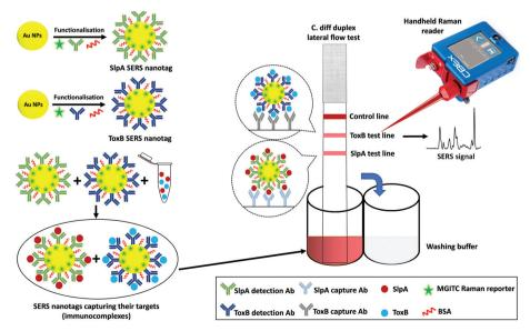
Fig. 1 Schematic representation for the duplex detection of SIpA and ToxB by SERS-based LFA
