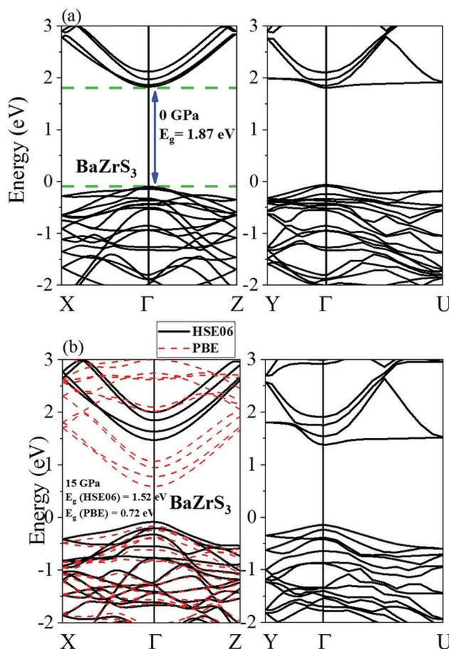
Fig. 6 Electronic band structure of BaZrS<sub>3</sub> at (a) 0 and (b) 15 GPa using HSE06 hybrid functional along with SOC. The black solid lines and red dashed lines denote the band structures obtained using HSE06 and PBE approximation respectively.
