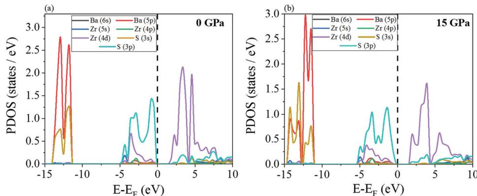
Fig. 9 PDOS of BaZrS<sub>3</sub> at (a) 0 and (b) 15 GPa using HSE06 hybrid functional along with SOC.
