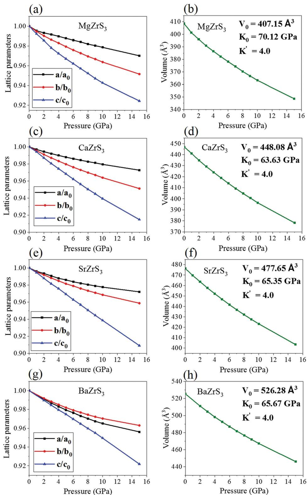
Fig. 4 (a) Evolution of lattice parameters with pressure and (b) equation of state of MgZrS<sub>3</sub>. (c) Evolution of lattice parameters with pressure and (d) equation of state of CaZrS<sub>3</sub>. (e) Evolution of lattice parameters with pressure and (f) equation of state of SrZrS<sub>3</sub>. (g) Evolution of lattice parameters with pressure and (h) equation of state of BaZrS<sub>3</sub>.
