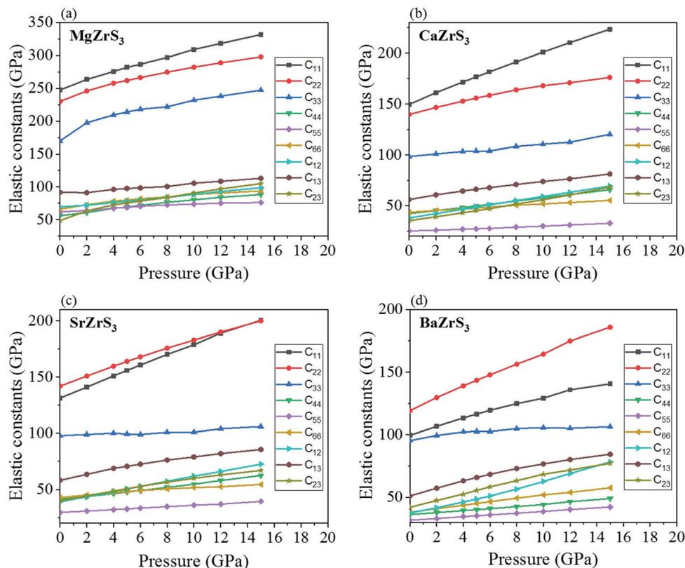
Fig. 3 Elastic constants vs. pressure for (a) MgZrS<sub>3</sub>, (b) CaZrS<sub>3</sub>, (c) SrZrS<sub>3</sub>, and (d) BaZrS<sub>3</sub>.
