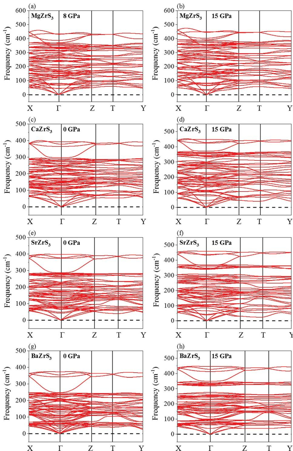
Fig. 2 Phonon dispersion curves for  $\text{MgZrS}_3$  at (a) 8 and (b) 15 GPa, for  $\text{CaZrS}_3$  at (c) 0 and (d) 15 GPa, for  $\text{SrZrS}_3$  at (e) 0 and (f) 15 GPa and for  $\text{BaZrS}_3$  at (g) 0 and (h) 15 GPa.
