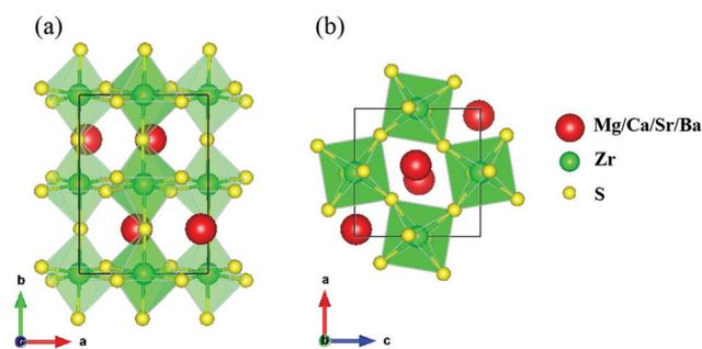
Fig. 1 Schematic of the *Pnma* AZrS<sub>3</sub> perovskites (A = Mg, Ca, Sr and Ba) viewed (a) along the *c*-axis and (b) along the *b*-axis.
