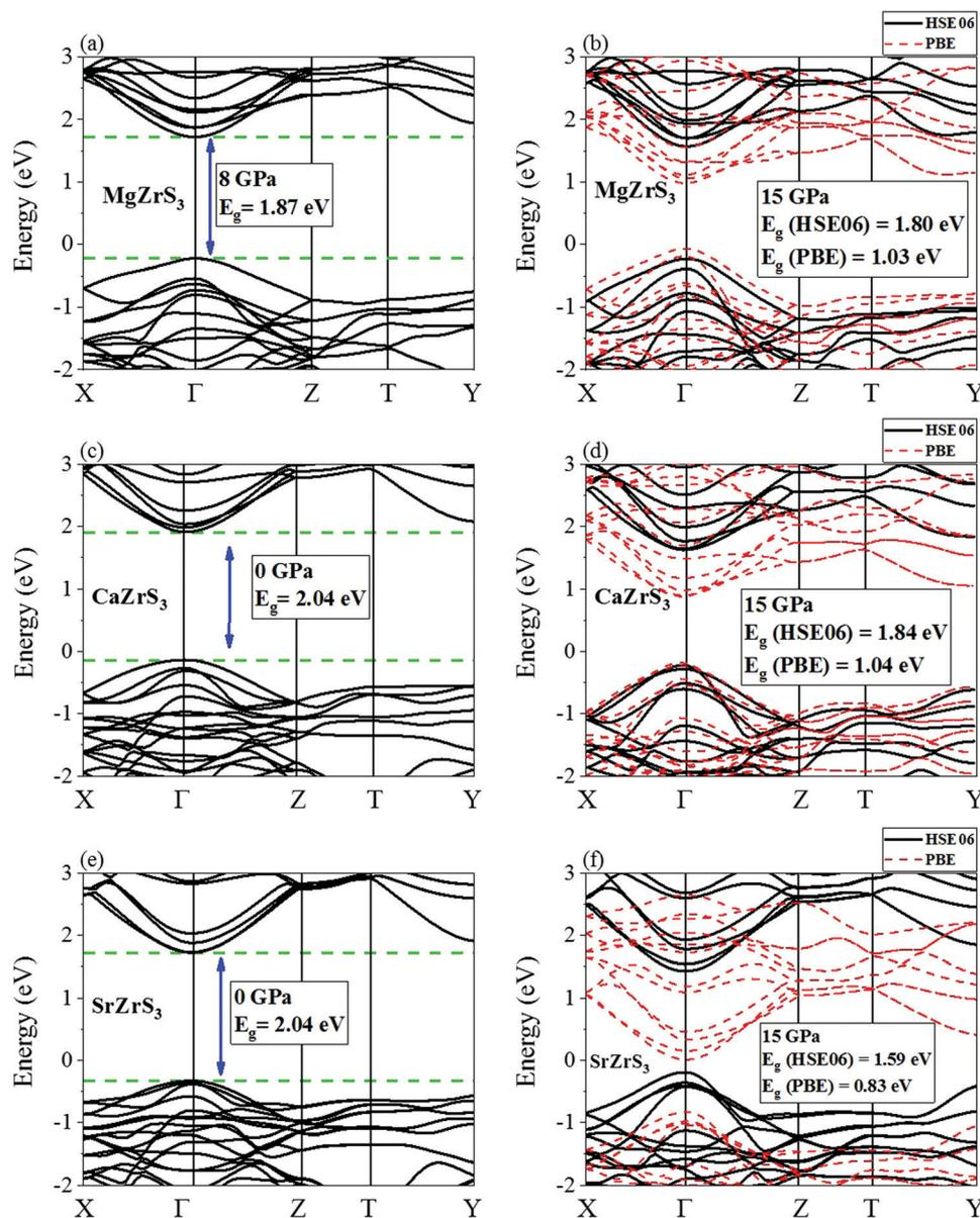
Fig. 5 Electronic band structure of  $\text{MgZrS}_3$  at (a) 8 and (b) 15 GPa, for  $\text{CaZrS}_3$  at (c) 0 and (d) 15 GPa and for  $\text{SrZrS}_3$  at (e) 0 and (f) 15 GPa. The black solid lines and red dashed lines denote the band structures obtained using HSE06 and PBE approximation respectively.
