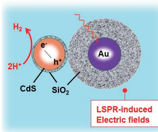
Fig. 4 LSPR-induced electric field immobilized on Au core–SiO 2 . Reproduced with permission from ref. 132.
