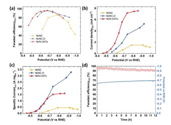
Fig. 4 The performance of the electrochemical CO<sub>2</sub> reduction on the as-prepared Ni/NC, Ni/NC-D, Ni/N-CNTs catalysts. (a) Faradaic efficiency, (b) geometric partial current density and (c) mass partial current density of CO as a function of potential; (d) faradaic efficiency and potential as a function of testing time for Ni/N-CNTs.
