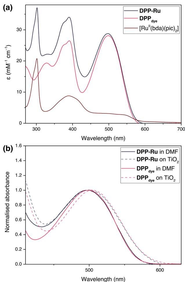
**Fig. 2** (a) UV-vis absorption spectra of  $\text{DPP}_{\text{dye}}$ ,  $[\text{Ru}^{\text{II}}(\text{bda})(\text{pic})_2]$  and  $\text{DPP-Ru}$  in DMF solution. (b) Normalised UV-vis spectra of  $\text{DPP}_{\text{dye}}$  and  $\text{DPP-Ru}$  on a  $\text{mTiO}_2$  film coated on a glass slide, and in DMF solution.
