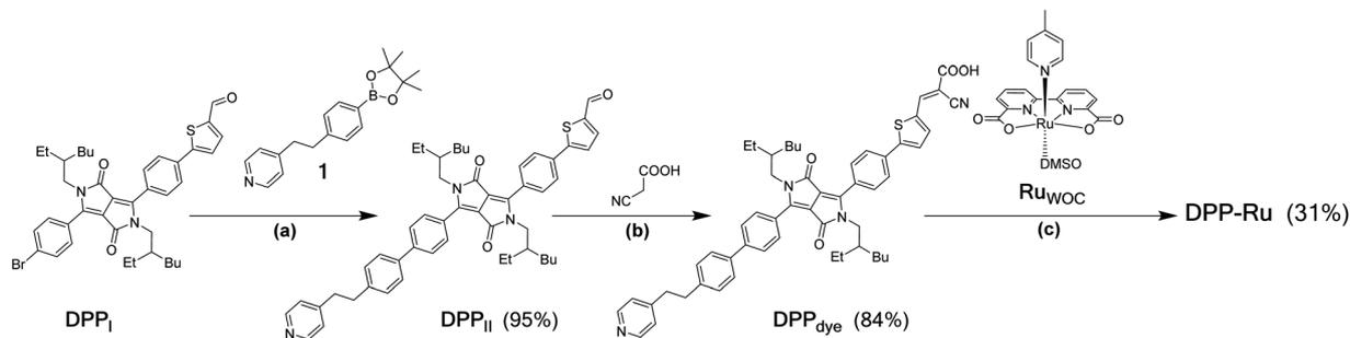
**Scheme 1** Synthesis of the water oxidising DPP-Ru dyad. Conditions: (a)  $[\text{Pd}(\text{PPh}_3)_4]$ ,  $\text{Na}_2\text{CO}_3$ , tetrahydrofuran/ $\text{H}_2\text{O}$  2 : 1,  $87^\circ\text{C}$ ,  $\text{N}_2$ , overnight; (b) piperidine, tetrahydrofuran, reflux,  $\text{N}_2$ , overnight; (c) MeOH, drops of triethylamine, reflux,  $\text{N}_2$ , overnight.
