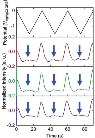
Fig. 5 Applied potential waveform (top) and corresponding individual fluorescence normalized intensity – time traces (bottom) for 3 different E-ZMWs containing 3  $\mu\text{M}$  redox-active AlexaFluor 488. Blue arrows indicate increase in fluorescence intensity at the negative end of the potential sweep.
