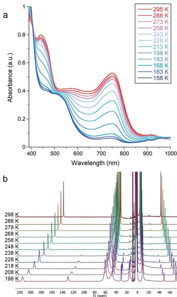
Fig. 3 (a) Variable temperature electronic absorption spectra of **4** in  $\text{Et}_2\text{O}$  under  $\text{N}_2$ . Absorbance values were corrected to account for the change in density of the solvent with temperature. (b) Variable temperature  $^1\text{H}$  NMR spectra of **4** in THF- $d_8$  under  $\text{N}_2$ .
