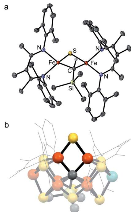
Fig. 2 (a) Crystal structure of [L<sup>Me</sup>Fe]<sub>2</sub>(μ-S)(μ-CHSiMe<sub>3</sub>) (2) with thermal ellipsoids shown at 50% probability. Color scheme: iron in orange, nitrogen in blue, carbon in gray, silicon in green, and sulfur in yellow. Hydrogen atoms have been omitted for clarity except on the alkylidene ligand. (b) Structural overlay of 2 with Fe<sub>2</sub>/Fe<sub>6</sub>/S<sub>2</sub>B/C rhomb in the FeMoco (nitrogenase crystal structure PDB 3U7Q).
