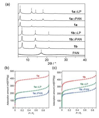
Fig. 3 (a) PXRD patterns of PAN, 1,  $1 \supset PAN$ , and  $1 \supset LP$ . (b and c)  $N_2$  adsorption isotherms of (b) 1a,  $1a \supset PAN$ ,  $1a \supset LP$ , (c) 1b,  $1b \supset PAN$ , and  $1b \supset LP$ .
