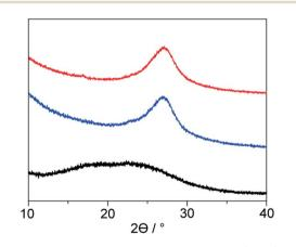
Fig. 6 PXRD patterns of LP prepared from neat PAN (black) and in 1a (red) and 1b (blue).
