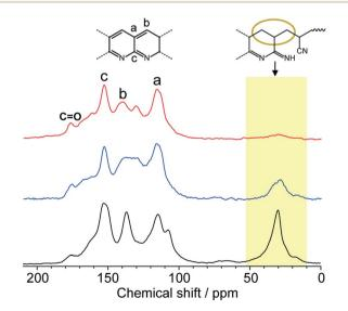
Fig. 5 Solid-state <sup>13</sup>C NMR spectra of LP prepared from neat PAN (black) and liberated from **1a** (red) and **1b** (blue).
