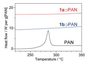
Fig. 8 DSC heating curves of 1a⊃PAN, 1b⊃PAN, and neat PAN.
