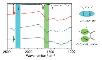
Fig. 4 IR spectra of neat PAN (black), LP liberated from **1a** (red) and **1b** (blue), and LP prepared from neat PAN (green).
