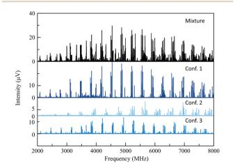
Fig. 2 The top spectrum (in black) shows the full MRR spectrum of the cyclohexanone reaction mixture at a temperature of  $165\,^{\circ}$ C. Beneath this are isolated MRR spectra of the three detected conformers of the major (3-substituted) product 3 in the arylation reaction.
