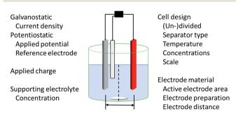
Fig. 3 Crucial parameters for reproducibility in electro-organic synthesis (batch-type).
