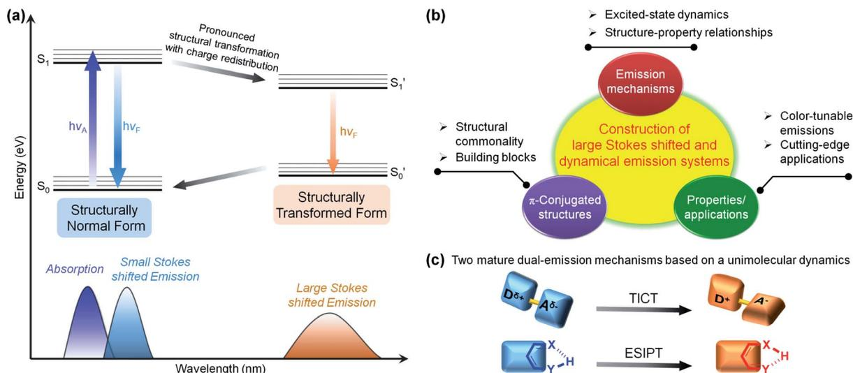
Fig. 1 (a) Jablonski diagram for the normal and transformed two-state model resulting in a large Stokes shift and dual fluorescence. (b) Route for the construction of a specific emission system and concept. (c) Illustrative schemes of two mature dual-emission mechanisms based on unimolecular dynamics: TICT and ESIPT.
