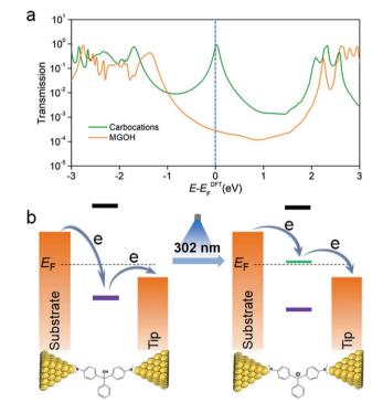
Fig. 4 (a) Transmission as a function of energy for the MGOH (orange) and carbocations (green) at room temperature.  $E_F$  is the Fermi level of the junction based on the DFT calculations. (b) Schematic diagram showing the position of the DFT resonances for carbocations respective to the two electrodes before and after light illumination.
