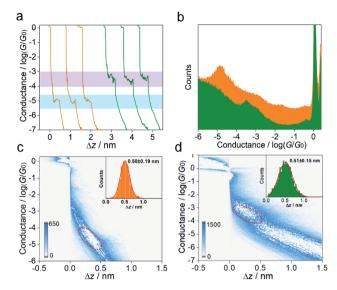
Fig. 2 (a) Typical conductance-distance traces of MGOH (orange) and carbocations (green). (b) 1D conductance-displacement histogram results constructed from thousands of individual traces for MGOH (vellow) and carbocations (green), 2D conductancedisplacement histograms versus the plateau relative displacement distributions of MGOH (c) and carbocations (d).
