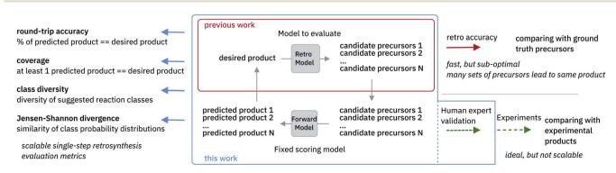
Fig. 2 Overview of single-step retrosynthesis evaluation metrics.
