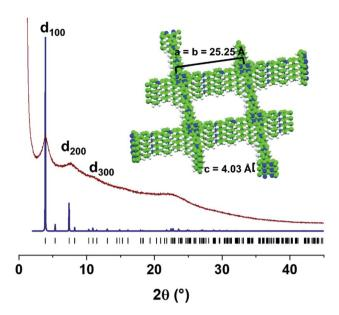
Fig. 3 Experimental PXRD pattern of the as-synthesized PV-COF (brown line) compared with the simulated pattern using the optimized crystal model (blue line), built in the P4-unit cell with a=b=25.25 Å, and c=4.03 Å. Inset: space-filling view of stacked layers along x and y-axes.
