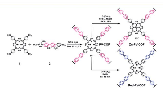
Fig. 1 Synthetic route to PV-COF through the Zincke reaction and its post-synthetic modifications by metalation of the porphyrin core (Zn-PV-COF) and chemical reduction of viologen units from a cationic to a neutral form (Red-PV-COF).
