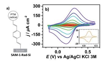
Fig. 2 (a) Sketch of SAM-1-Rad-Si. (b) Cyclic voltammograms under red light illumination of SAM-1-Rad-Si at different scan rates (0.1, 0.2, 0.4, 0.6, 1, 2, 4, 6 and 10 V s<sup>-1</sup>, from brown to purple) in CH<sub>3</sub>CN + 0.1 M Bu<sub>4</sub>NClO<sub>4</sub>. The inset shows comparative CVs at 0.4 V s<sup>-1</sup> in the dark (dashed line) and under illumination (solid line).
