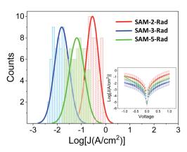
Fig. 6 Histograms and Gaussian fits of log | J | at 1 V for junctions Au<sup>TS</sup>/ SAM-2,3 and 5-Rad//GaO<sub>x</sub>/EGaIn. Inset: Plots of mean log|J| versus E(V)
