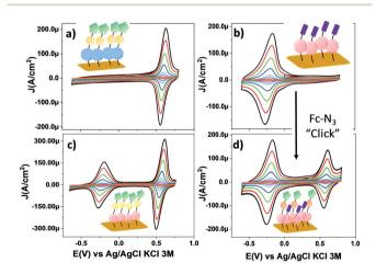
Fig. 4 CV curves of SAMs on gold: (a) SAM-3-H, (b) SAM-2-Rad, (c) SAM-3-Rad and (d) SAM-5-Rad in  $CH_2Cl_2+0.2$  M  $Bu_4NPF_6$  at different scan rates (0.05, 0.1, 0.25, 0.5, 1, 2, 3 and 4 V s $^{-1}$ ). The color code used for SAMs is the same as that used in Scheme 1. (Blue) PTM  $\alpha H_1^2$  (magenta) PTM radical; (yellow) triazole ring; (green) Fc and (violet) terminal alkyne moieties.
