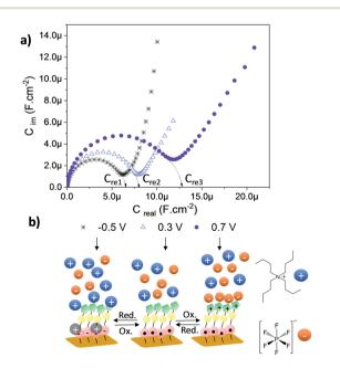
Fig. 5 (a) Cole-Cole plots recorded for the SAM-3-rad at different applied potentials to obtain three different redox states. The electrolytic medium (CH<sub>2</sub>Cl<sub>2</sub> + 0.2 M Bu<sub>4</sub>NPF<sub>6</sub>) was used and the frequency was varied from 100 kHz to 0.1 Hz with a 20 mV amplitude. (b) Scheme of the three different interfaces at the specific applied voltage.
