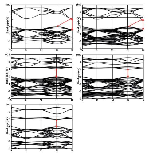
Fig. 5 Calculated band structures of double perovskites along the X-R-M-G-R path for (a)  $Cs_2Te_{0.75}Ti_{0.25}I_{0}$ , (c)  $Cs_2Te_{0.50}Ti_{0.50}I_{0}$ , (d)  $Cs_2Te_{0.25}Ti_{0.75}I_6$ , and (e)  $Cs_2TiI_6$ .
