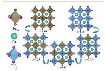
Fig. 1 The optimized structures of the  $Cs_2Te_{1-x}Ti_xI_6$  solid solutions.
