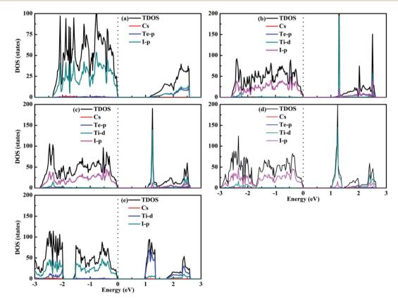
Fig. 7 Density of states of (a)  $Cs_2Tel_6$ , (b)  $Cs_2Te_{0.75}Ti_{0.25}l_6$ , (c)  $Cs_2Te_{0.50}Ti_{0.50}l_6$ , (d)  $Cs_2Te_{0.25}Ti_{0.75}l_6$ , and (e)  $Cs_2Til_6$ .
