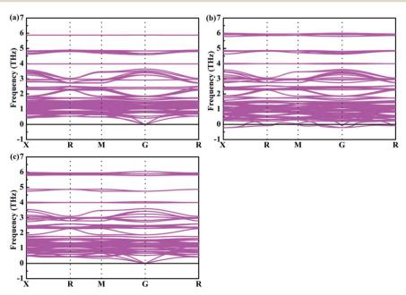
Fig. 4 Phonon spectrum of (a)  $Cs_2Te_{0.75}Ti_{0.25}I_6$ , (b)  $Cs_2Te_{0.50}Ti_{0.50}I_6$ , and (c)  $Cs_2Te_{0.25}Ti_{0.75}I_6$ .
