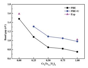
Fig. 6 Experimental and theoretical band gap trends with different methods of  $Cs_2Te_{1-x}Ti_xI_6$ .
