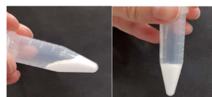
Fig. 1 DES in water emulsion (30 : 70 volume ratio) stabilised by 1.5 wt% OCNF after more than 200 days at room temperature.
