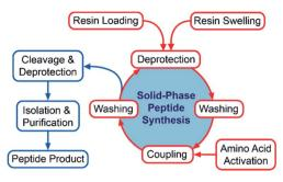
Fig. 1 Overview of the SPPS cycle and subsequent deprotection, work-up and purification steps. The present review focuses on technical aspects of the SPPS cycle (shown in red) while cleavage, deprotection, isolation and purification steps (shown in blue), are only briefly touched upon.
