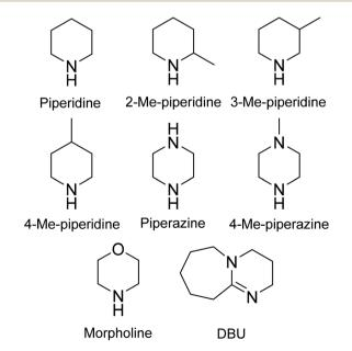
Fig. 3 Chemical structures of organic bases investigated for Fmocremoval in SPPS.
