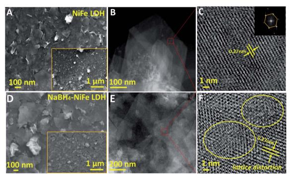
Fig. 2 Morphology and structure characterizations. SEM (A and D), TEM (B and E) and HRTEM (C and F) images of NiFe LDH (A-C) and NaBH<sub>4</sub>-NiFe LDH (D-F). The yellow circles in F indicated lattice distortions.
