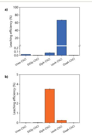
Fig. 2 Effect of the hydrogen-bond donor type on the leaching efficiency of (a) YOX lamp phosphor and (b) HALO lamp phosphor. The leaching conditions are: H<sub>2</sub>O vol% = 10;  $T=80~^{\circ}\text{C}$ ; t=48~h; L/S = 10 and 500 rpm.
