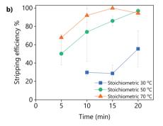
Fig. 12 Stripping efficiency obtained by the addition of pure oxalic acid to (a) LevA-ChCl and (b) levulinic acid PLS, as a function of the amount of oxalic acid, mixing temperature and time. The leaching conditions are:  $H_2O$  vol% = 30; T = 80 °C; t = 48 h; L/S = 10; 500 rpm.
