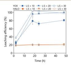
Fig. 10 Effect of the L/S ratio and leaching time on the leaching efficiency of a real lamp phosphor waste using the ionic liquid [Hbet] [NTf<sub>2</sub>]. The leaching conditions are:  $H_2O$  vol% = 5; T = 80 °C; 500 rpm.
