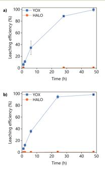
Fig. 5 Effect of the leaching time on the leaching efficiency of YOX and HALO using (a) LevA–ChCl and (b) levulinic acid. The leaching conditions are: T = 80 °C; L/S = 10; H<sub>2</sub>O vol% = 30; and 500 rpm.
