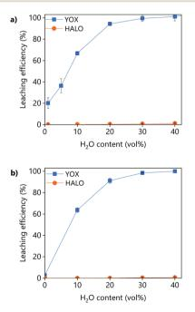
Fig. 4 Effect of the water content on the leaching efficiency of YOX and HALO using (a) LevA–ChCl and (b) levulinic acid. The leaching conditions are: T=80 °C, t=48 h, L/S = 10 and 500 rpm.
