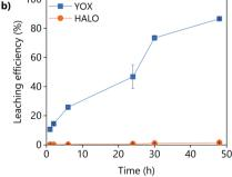
Fig. 7 Effect of the mixing time on the leaching efficiency of a synthetic lamp phosphor mixture using (a) LevA–ChCl and (b) levulinic acid. The leaching conditions are:  $H_2O$  vol% = 30; T=80 °C; L/S = 10: 500 rpm.
