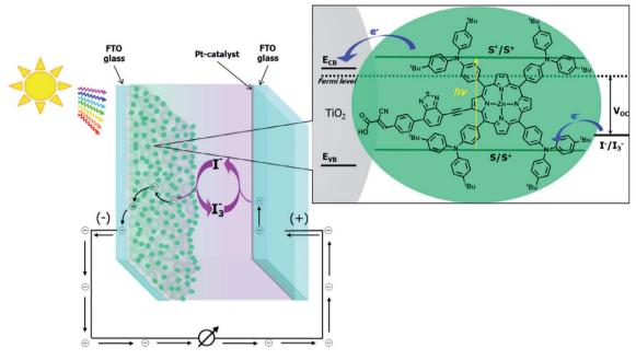
Fig. 21 Working principle of the universal design of DSSC. Reproduced with permission from ref. 212, copyright 2018, Elsevier.
