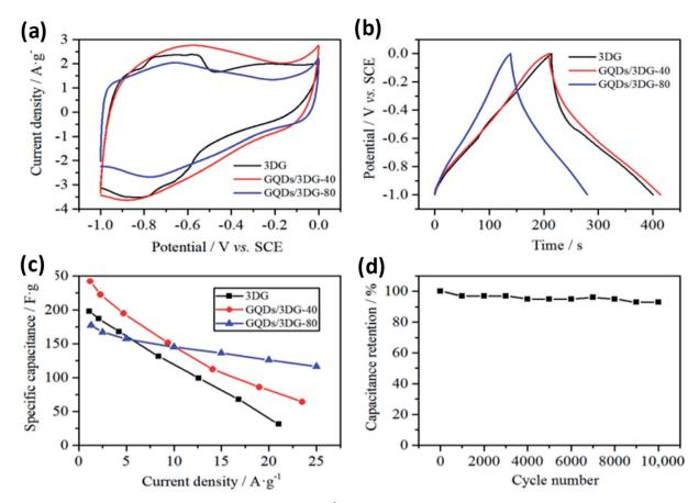
Fig. 18 (a) Cyclic voltammetry curve at a scan rate of 10 mV s<sup>-1</sup> (b) charge/discharge curves at different current densities with different compositions, respectively (c) specific capacitance versus current densities and (d) cycling stability at a current density of 24 A g<sup>-1</sup> for the composite material. Adapted from ref. 183, copyright 2019, MDPI publications.
