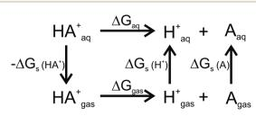
Fig. 1 Thermodynamic cycle used for p $K_a$  calculations.  $\Delta G_{gas}$  free energy of deprotonation in gas-phase;  $\Delta G_s$  solvation free energy;  $\Delta G_{aq}$ free energy of deprotonation in aqueous solution.
