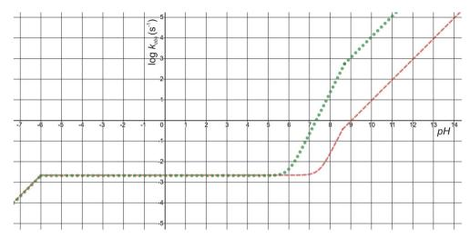
Fig. 6 The pH-dependence of predicted observed reaction rate constant for noradrenaline (red interrupted line) and adrenaline (green dotted line) o-quinone cyclization reaction applying the experimental  $pK_a$  values from Table 2.
