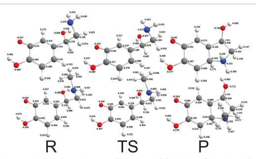
Fig. 5 Optimized geometries and atomic charges of the reactants (R), transition state (TS) and products (P) of noradrenaline (top) and adrenaline (bottom) o-quinone with protonated quinone group cyclization reaction. Reactants are catecholamine o-quinone with protonated quinone group and unprotonated amino group. Products are cyclized single charged catecholamine o-quinone. Carbon atoms are represented with gray, oxygen atoms red, hydrogen atoms white and nitrogen atoms with blue color.
