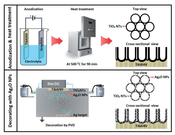
Fig. 3 Schematic representation of the anodization setup and the development of  $TiO_2$  NTs as well as PVD decoration of  $Ag_2O$  NPs on the nanotubular layer. <sup>122</sup>
