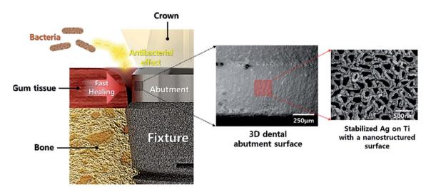
Fig. 5 Antibacterial and bioactive properties of stabilized silver on titanium with a nanostructured surface for dental implants. 128
