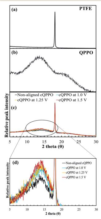
Fig. 14 XRD patterns: (a) the porous PTFE, (b) QPPO membrane and (c) cQPPO membranes; (d) comparison of peak intensity according to applied intensity of the electric field.
