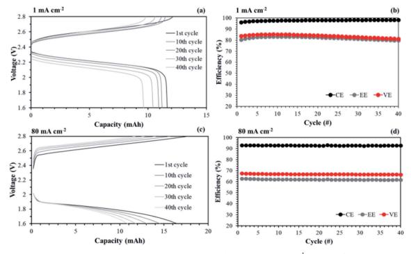
Fig. 16 Comparison of performances in a single cell using  $0.05 \text{ M V}(\text{acac})_3/\text{TEABF}_4$  at  $60 \text{ mL min}^{-1}$ : (a) charge/discharge curves and (b) efficiencies by applying AHA membrane; (c) charge/discharge curves and (b) efficiencies by introducing the aligned cQPPO membrane at 1.5 V.
