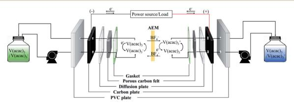
Fig. 5 Diagram of the operating NAVRFB system; solid and dashed lines represent the charge/discharge process, respectively.
