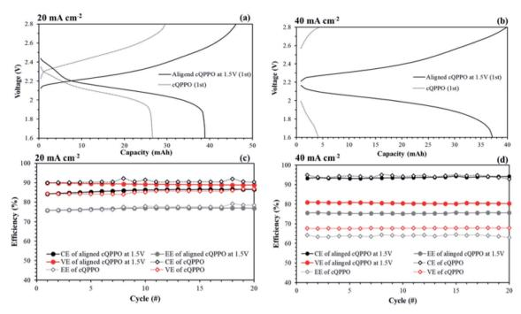
Fig. 15 Comparison of performances in a single cell using  $0.05 \text{ M V}(\text{acac})_3/\text{TEABF}_4$  at  $60 \text{ mL min}^{-1}$ : (a) charge/discharge curves at (a) 20 and (b) 40 mA cm<sup>-2</sup>; efficiencies at (c) 20 and (d) 40 mA cm<sup>-2</sup> by applying the non-aligned and aligned cQPPO membrane.
