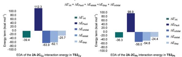
Fig. 7 (a) Distortion/interaction model (kcal mol<sup>-1</sup>) and (b) energy decomposition analysis of TS2<sub>Cy</sub> and 2TS<sub>Ph</sub>.  $\Delta G^{\ddagger}$  and  $\Delta E_{TS}$  is calculated at the level of B3PW91/6-31G(d) planted in the Gaussian 16 program.  $^{26}$   $\Delta E'_{int}$  is dissected into chemically meaningful terms according to the ETS-NOCV calculations at the level of B3LYP-D3/DZP planted in the Amsterdam density functional (ADF) package.<sup>24</sup>
