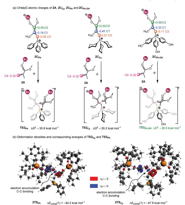
Fig. 8 (a) CHelpG atomic charge  $^{25}$  in 2A,  $^{2}C_{Ph}$ ,  $^{2}C_{Cy}$  and  $^{2}C_{Ph-OH}$ ; (b) leading deformation densities and corresponding energies for  $^{25}C_{Ph}$  and  $2TS_{Cy}$ . The red color denotes charge depletion and the blue color represents charge accumulation ( $|\Delta \rho| = 0.004$  a.u. for all the density surfaces).
