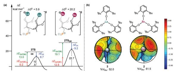
Fig. 5 (a) Distortion/interaction analyses (kcal mol<sup>-1</sup>) of 3TS<sub>DE</sub> and 2TS<sub>DE</sub>; (b) topographical steric maps of catalysts 3 and 2.
