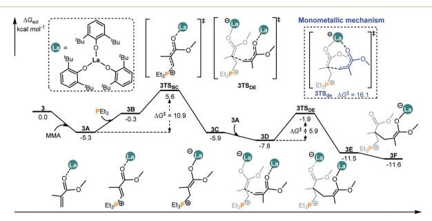
Fig. 4 Computed energy profiles for the 3/PEt<sub>3</sub> mediated (intermolecular RE/P systems) bimetallic pathway for MMA enchainment. Free energies (kcal mol<sup>-1</sup>) are relative to isolated reactants.
