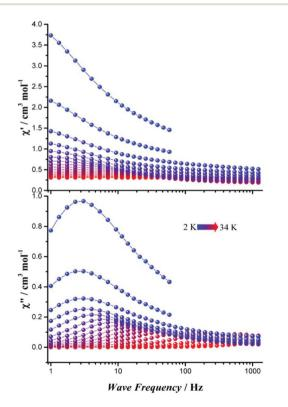
Fig. 3 Frequency-dependent in-phase (upper) and (lower) ac susceptibility of 8 in zero static field.
