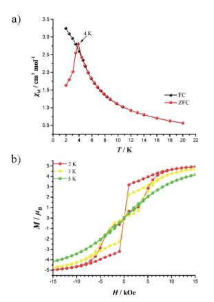
Fig. 4 (a) FC (black) and ZFC (red) magnetization plots for 8. (b) Magnetic hysteresis loops for 8 between 2 K and 5 K with a field sweeping rate of 12 Oe s<sup>-1</sup>.
