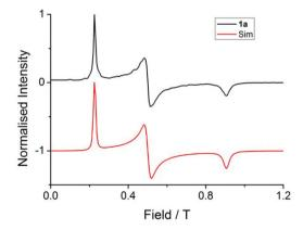
Fig. 2 Q-Band EPR measurement at 33.995818 GHz collected at 5 K on the 5% diluted 1a  $[Y{5\%Er}_2(HMeQ^*)_2(NO_3)_6]$  (black) with the fitted spectrum (red), following the procedure outlined in previous work.<sup>27</sup> g-Values are in Table 1, linewidths:  $lw_1 = 1.7$ ,  $lw_2 = 2.3$  and  $lw_3 = 1.3$ GHz.
