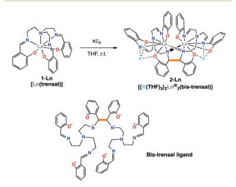
Scheme 2 Synthesis of [{K(THF)<sub>3</sub>}<sub>2</sub>Ln<sub>2</sub>(bis-trensal)], 2-Ln, Ln = Nd, Sm.
