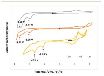
Fig. 4 Cyclic voltammogram of complexes 1-Nd (grey), 1-Sm (orange) and 1-U (yellow) from ref. 10c in  $\sim$ 0.1 M [Bu<sub>4</sub>N][PF<sub>6</sub>] THF solution at a 100 mV s<sup>-1</sup> scan rate.
