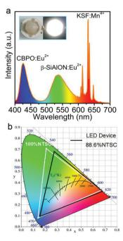
Fig. 5 (a) Emission spectrum of w-LED fabricated by mixing blue  $Ca_2Be_2(PO_4)_2$ :  $Eu^{2+}$ , green  $\beta$ -Sialon:  $Eu^{2+}$ , and red  $K_2SiF_6$ :  $Mn^{4+}$  on a near-UV LED chip (380 nm), under 30 mA driving current. The inset shows photographs of the w-LED device taken under daylight and when it is in operation. (b) Color gamut of the NTSC standard (white triangle) and the as-fabricated w-LED device (black triangle).
