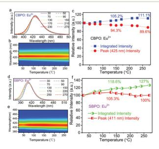
Fig. 4 Temperature-dependent emission spectra of (a and b)  $Ca_2Be_2(PO_4)_2$ :  $Eu^{2+}$  and (d and e)  $Sr_2Be_2(PO_4)_2$ :  $Eu^{2+}$  phosphors in the temperature range of 30-270 °C. Temperature-dependent normalized integrated emission spectra and maximum emission peak intensity of (c)  $Ca_2Be_2(PO_4)_2$ :  $Eu^{2+}$  and (f)  $Sr_2Be_2(PO_4)_2$ :  $Eu^{2+}$  phosphors.
