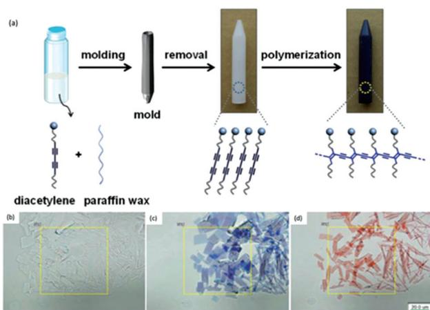
**Fig. 21** (a) Schematic diagram of the PDA-paraffin wax composite sensor synthesis. Optical microscopic images of PDA-wax composite (b) before 254 nm UV irradiation, (c) after irradiation, and (d) after heat treatment at 55 °C for 10 seconds. Scale bars are 20  $\mu$ m. Reproduced from ref. 69 with permission from WILEY-VCH Verlag GmbH & Co., copyright [2016].
