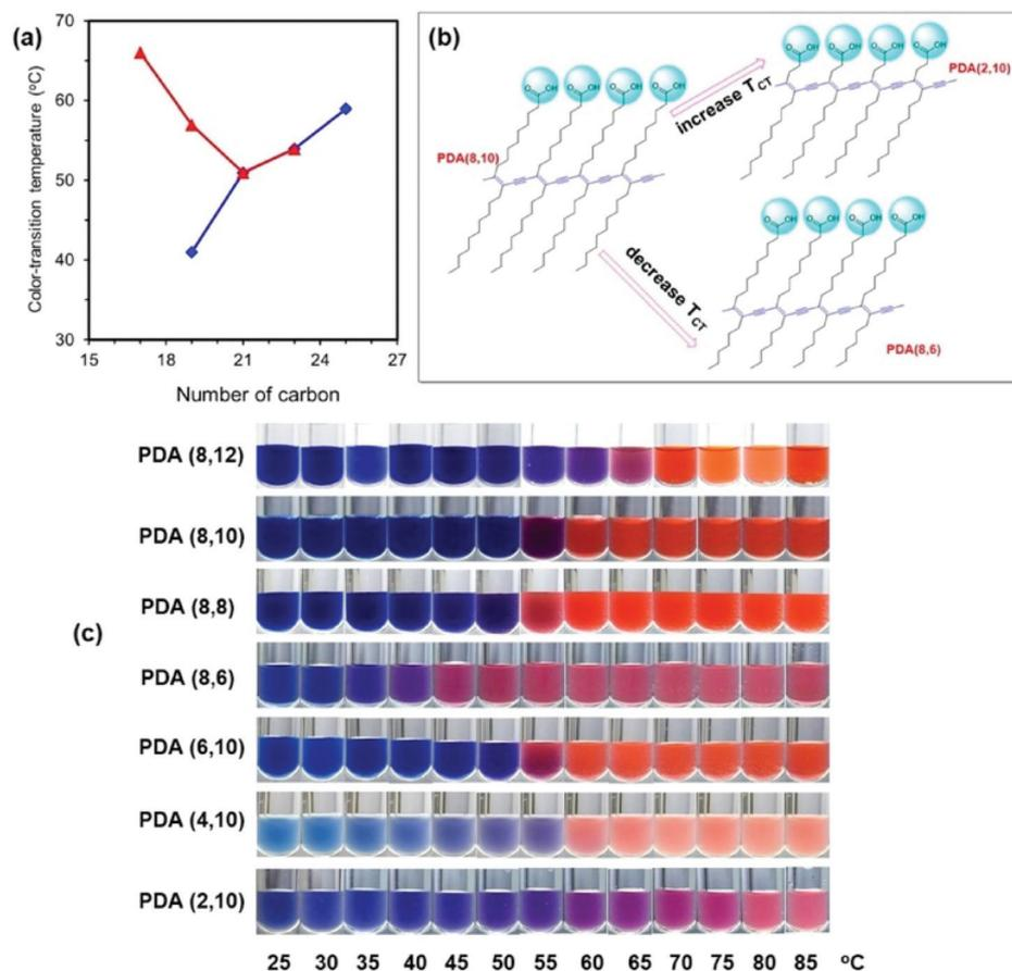
Fig. 8 (a) Plots of color transition temperature ( $T_{CT}$ ) versus number of carbon within the repeating unit of PDAs. Symbols are for ( $\blacklozenge$ , blue) PDA(8,y) and ( $\blacktriangle$ , red) PDA(x,10). (b) The opposite change of  $T_{CT}$  when the alkyl segments at different regions are shortened. (c) Color photographs of PDAs in aqueous suspension taken upon increasing temperature. Reproduced from ref. 41 with permission from Elsevier, copyright [2018].
