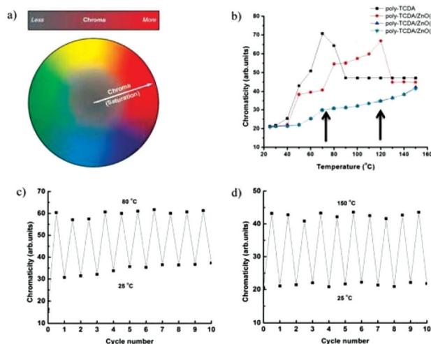
**Fig. 16** (a) Schematic showing chromaticity distribution from dull to vivid. (b) Chromaticity versus temperature plots for TCDA and TCDA/ZnO composites. (c) Chromaticity of TCDA/ZnO (5 wt%) as a function of thermal cycle. (d) Chromaticity of TCDA/ZnO (15 wt%) as a function of thermal cycle. Reproduced from ref. 58 with permission from the American Chemical Society, copyright [2013].
