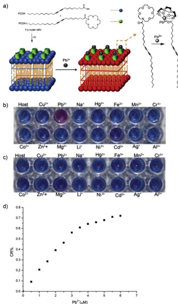
**Fig. 11** (a) The synthesis and binding mechanism of poly-PDA-L with Pb<sup>2+</sup>. PCDA-L and PCDA was mixed at 3 : 7 molar ratio. Digital images of the colorimetric responses of (b) poly-PDA-L and (c) pure PDA vesicles towards various metal ions (10 μM) in HEPES buffer. (d) Colorimetric response (CR%) of poly-PDA-L at different Pb<sup>2+</sup> concentrations in HEPES buffer. Reproduced from ref. 48 with permission from Elsevier, copyright [2015].
