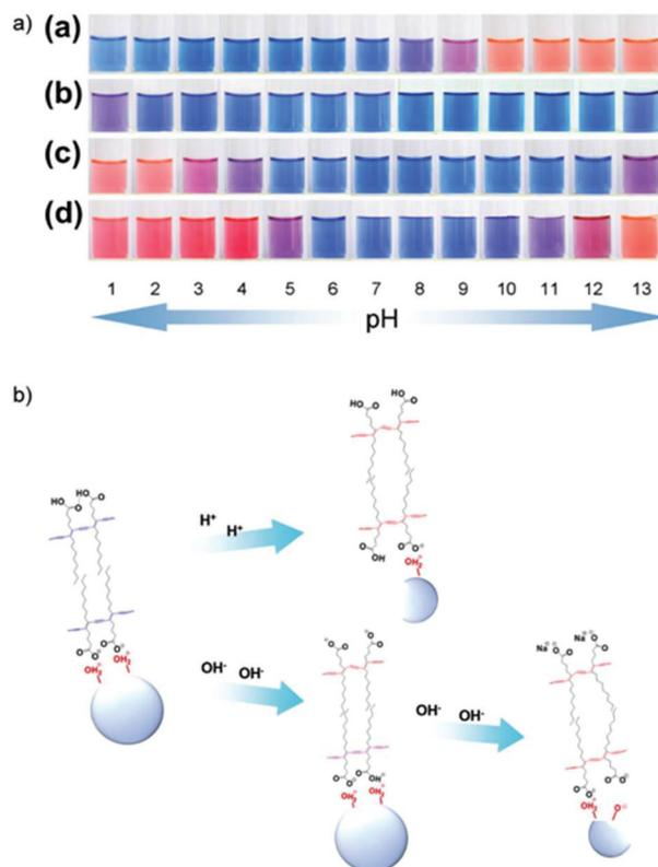
**Fig. 18** (a) Photographs of aqueous suspensions of (a) pure poly(TCDA), (b) poly(PCDA)/ZnO (c) poly(TCDA)/ZnO, and (d) poly(HDDA)/ZnO nanocomposites taken at different pH. (b) The ZnO dissociation model and color change mechanism of PDA/ZnO nanocomposites at low and high pH. Reproduced from ref. 61 with permission from Elsevier, copyright [2014].
