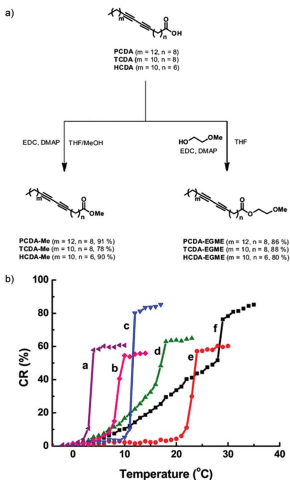
**Fig. 10** (a) Schematic diagram of the preparation of diacetylene monomers to produce low temperature thermochromic PDA nanosensors. (b) Colorimetric response (CR) plot as a function of temperature of PDAs functionalized with ester moieties; (a) HCDA-EGME, (b) HCDA-Me, (c) TCDA-EGME, (d) TCDA-Me, (e) PCDA-EGME, (f) PCDA-Me. Reproduced from ref. 47 with permission from the American Chemical Society, copyright [2016].
