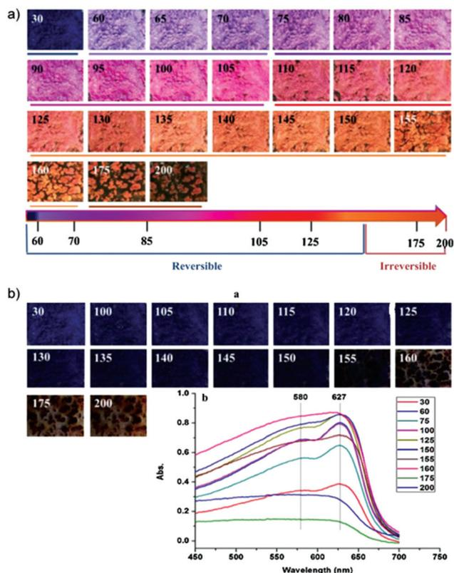
**Fig. 9** (a) Photographs of PDA-urea at temperatures ranging from 30 to 200 °C post-2 minutes equilibration. The color transition path with its reversibility upon heating is represented as the rainbow line. (b) Photographs of PDA-urea powders at room temperature after cooling. Reproduced from ref. 46 with permission from Elsevier, copyright [2017].
