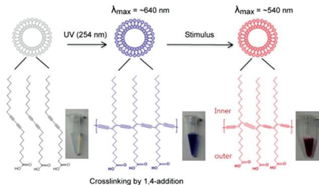
**Fig. 1** Chemical structure of polydiacetylene and its chromatic properties. Polymerized backbone of vesicles and blue-to-red color transition is shown. Adapted from ref. 23 with permission from MDPI, copyright [2012].
