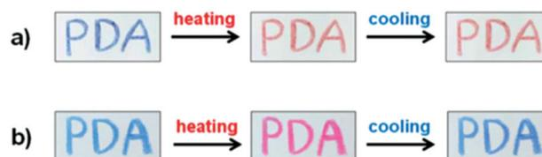
**Fig. 22** Handwritten PDA image on paper derived from (a) PDA-wax when heated at 70 °C for 30 seconds then cooled and (b) colorimetric response of PDA-mBzA-wax heated to 120 °C and cooled. Reproduced from ref. 69 with permission from WILEY-VCH Verlag GmbH & Co., copyright [2016].
