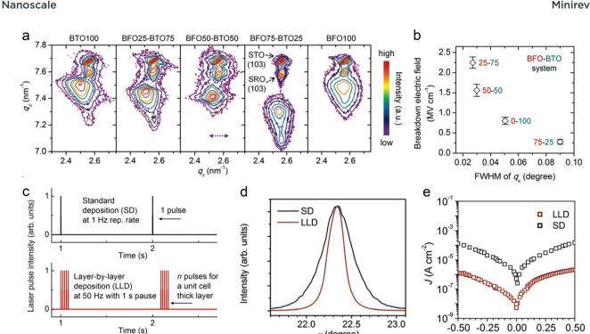
Fig. 3 (a) RSM of BFO-BTO dielectric films around the (103) peaks.<sup>47</sup> (b) Breakdown field of the BFO-BTO films as a function of the FWHM of  $q_x$  of the RSM in (a). 47 Copyright © 2018, Elsevier. (c) Schematic comparison of the LLD and SD strategies for pulsed laser film deposition. 51 (d) Rockingcurve ( $\omega$  scan) and (e) leakage current of the 25% BFO + 75% BTO films fabricated by SD and LLD strategies, respectively. 51 Copyright © 2020, Elsevier.
