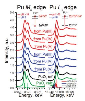
Fig. 3 Pu  $M_4$  and  $L_3$  HERFD experimental data. Data recorded for six  $PuO_2$  NPs samples and compared with a  $PuO_2$  reference and theoretical calculations, using AIM approximation (left) and FEFF code (right). The density of states is plotted at the bottom for clarity.
