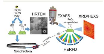
Fig. 1 The schematic illustration of the research methodology applied to PuO<sub>2</sub> NPs studies. PuO<sub>2</sub> NPs synthesized from different precursors (Pu(III), Pu(IV) and Pu(V)) and at pH 8 and pH > 10 were analysed with HRTEM and various synchrotron techniques (EXAFS, XRD, HEXS and HERFD)
