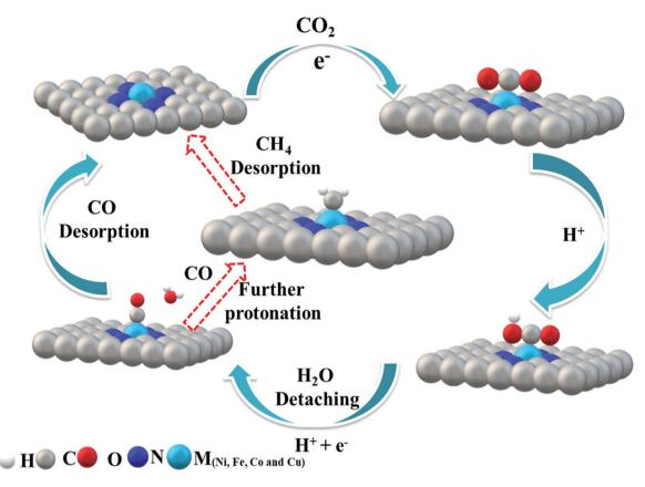
Fig. 7 Proposed reaction paths for  $CO_2$  electroreduction by M-N-C. Fe-N-C follows the red arrow to further undergo protonation to give methane (CH<sub>4</sub>).
