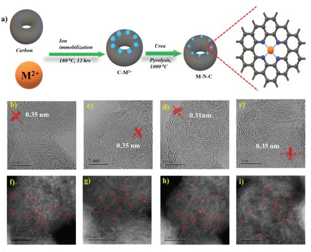
Fig. 1 Schematic of the synthesis process of the M-N-C catalyst (a). Aberration-corrected bright-field STEM image of (b) Ni-N-C, (c) Fe-N-C, (d) Co-N-C and (e) Cu-N-C and their respective aberration-corrected HAADF-STEM images (f-i).
