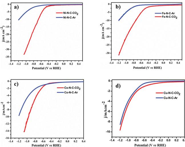
Fig. 4  $CO_2$  reduction reaction activities. Linear sweep voltammetry of (a) Ni–N–C, (b) Fe–N–C, (c) Co–N–C and (d) Cu–N–C in  $CO_2$ -saturated 0.1 M KHCO<sub>3</sub> (red lines) and in N<sub>2</sub>-saturated 0.1 M KHCO<sub>3</sub> (blue lines) at 5 mV s<sup>-1</sup> in the cathodic direction.
