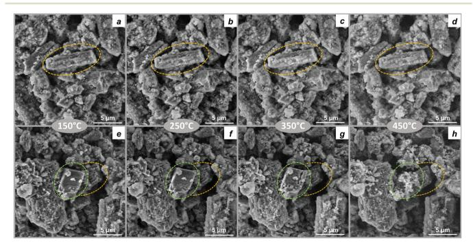
Fig. 6 In situ SEM images obtained while heating (a-d) HM and (e-h) HM-20NaNO<sub>3</sub> from 100 °C to 450 °C in 46 Pa of N<sub>2</sub>. The areas highlighted in yellow in Fig. 6a-h shows the HM particle agglomerates, while areas highlighted in green in Fig. 6e-h emphasizes the thermal evolution of typical NaNO<sub>3</sub> particle.
