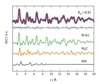
Fig. 8 PDF refinement of Ni(BDC)(PNO) decomposed at 375  $^{\circ}$ C in He with three phases (Ni<sub>fcc</sub>, Ni<sub>3</sub>C and NiO). Blue open circles represent the experimental PDF and red line the calculated PDF. The grey line in the offset shows the difference between experimental and calculated PDF.
