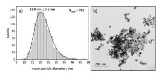
Fig. 9 (a) Particle size distribution of Ni(BDC)(PNO) decomposed at 375 °C in 5% H<sub>2</sub>/He and (b) corresponding TEM image of the sample.
