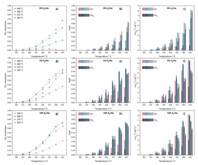
Fig. 12 CO<sub>2</sub> conversions (a, d and g), stacked CH<sub>4</sub> and CO yields (b, e and h) and stacked productivities of CH<sub>4</sub> and CO normalized to the molar Ni content (c, f and i) of Ni(BDC)(PNO) decomposed at temperatures of 350 °C (red), 375 °C (blue), 400 °C (green) and 500 °C (purple) in 0% (a–c), 5% (d–f) and 10% H<sub>2</sub>/He (g–i) atmospheres.
