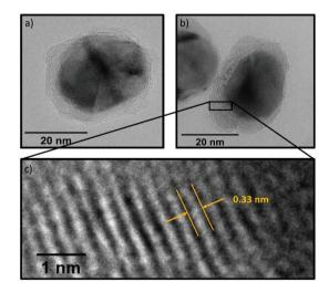
Fig. 10 (a) TEM of a polycrystalline particle after decomposition at 400 °C in 10%  $\rm H_2$  with graphitic shell. (b) TEM of a particle after decomposition at 500 °C in 10%  $\rm H_2$ , no twinning is visible. (c) Zoom into carbon shell, revealing a layered carbon structure with 0.33 nm interlayer spacing.
