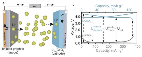
Fig. 1 (a) Schematic illustrating the operating principle of a rechargeable LIB with graphite as the anode material and LiCoO<sub>2</sub> as the cathode material (b) Galvanostatic charge/discharge curves of LiCoO2 and graphite measured in combination with metallic lithium as counter and reference electrodes (half-cell configuration).
