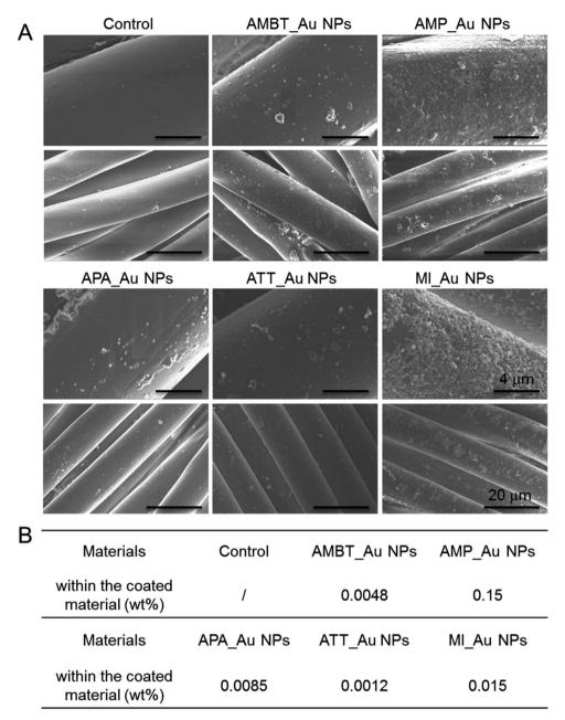
Fig. 4 Characterization of the control fabrics and N\_Au NP-coated fabrics. (A) SEM images of control fabrics or fabrics coated with different ligands. The scale bar was 4 μm or 20 μm. (B) ICP analysis of the coated fabrics showing the concentration of N\_Au NPs within the different surfaces. The standard deviation of the ICP results corresponded to 1%
