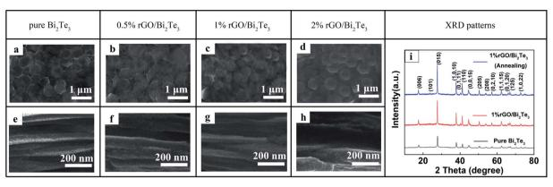
Fig. 1 Surface and cross-sectional SEM images of  $Bi_2Te_3$  nanoplate films with different mass ratio of rGO nanosheets: (a) and (e) pure  $Bi_2Te_3$ , (b) and (f) 0.5% rGO/ $Bi_2Te_3$ , (c) and (g) 1% rGO/ $Bi_2Te_3$ , and (d) and (h) 2% rGO/ $Bi_2Te_3$ ; (i) XRD patterns of the pure  $Bi_2Te_3$  and 1% rGO/ $Bi_2Te_3$  composites films before and after annealing.
