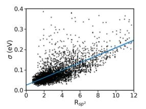
Fig. 4 Correlation between  $\sigma$  and  $R_{\rm sp^2}$  for the considered database of molecular semiconductors.
