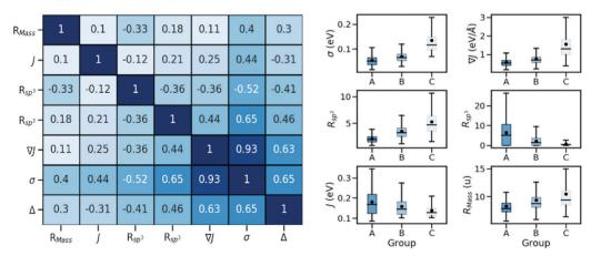
Fig. 2 (left) Spearman's rank correlation between parameters. (right) Variation range of parameters correlated with the relative dynamic disorder (i.e.  $\sigma$ ,  $\nabla J$ ,  $R_{\rm Sp^2}$ ,  $R_{\rm Sp^3}$ , J and  $R_{\rm Mass}$ ) among defined categories of A, B, and C depicted on a series of "box plots". The box limits represent the first ( $Q_1$ ) and third quartiles ( $Q_3$ ), with a line and a small circle representing the median and the mean value, respectively.
