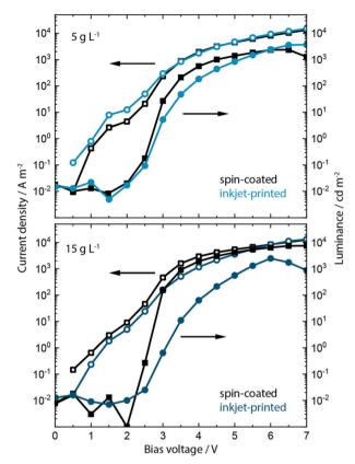
**Fig. 4** The J/V/L characteristics of PeLEDs fabricated on PEDOT:PSS blended with a low 5 g L<sup>-1</sup> KCl content (a) and high 15 g L<sup>-1</sup> KCl content (b) indicate the two different optimums depending on the process – for low KCl content devices incorporating the inkjet-printed active layer outperform those incorporating the spin-coated ones. For higher KCl content, it is *vice versa*.
