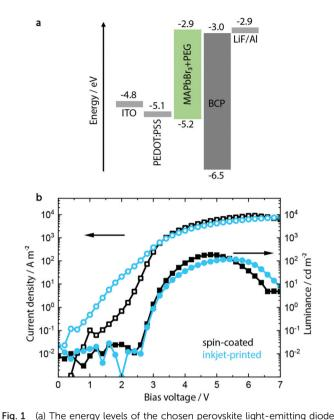
(PeLED) device architecture permit ohmic contact between both the hole and electron injection layer and the semiconducting perovskite. (b) Current density/voltage/luminance characteristics show similar device parameters for the spin-coated and inkjet-printed PeLEDs without KCl as additive.
