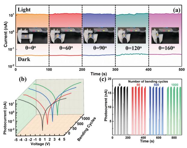
Fig. 4 (a) Output currents of the device with different bending angles under dark and light illumination with a light intensity of 0.2 mW cm<sup>-2</sup> at a bias voltage of 5 V. The insets are the corresponding optical images of the device under five bending states.  $\theta$  is the bending angle. (b) I-V and (c) I-t curves of the device under different bending cycles.
