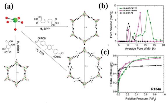
Fig. 4 (a) Schematic representation of the  $Ni^{2+}$  node, organic bridging ligands, and corresponding structures (viewed along the c-axis) of the poreexpanded Ni-MOF-74 analogues. (b) Pore size distributions. (c) R134a pure gas adsorption isotherms at 298 K; the black, magenta, and green curves correspond to Ni-MOF-4, Ni-BPP, and Ni-TPP, respectively.<sup>40</sup> Reproduced from ref. 40 with permission from The Royal Society of Chemistry.
