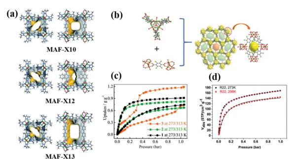
Fig. 3 (a) The pore structure of MAF-X10, MAF-X12 and MAF-X13 viewed along two characteristic directions. (b) The trimeric Fe<sub>3</sub>O cluster, tcdc<sup>2-</sup> coordination mode and packing diagram along the c axis of LIFM-26. (c) and (d) R22 adsorption isotherms of MAF-X10, MAF-X12, MAF-X13 and LIFM-26, respectively.<sup>37,39</sup> Reproduced from ref. 37 and 39 with permission from The Royal Society of Chemistry & Wiley-VCH.
