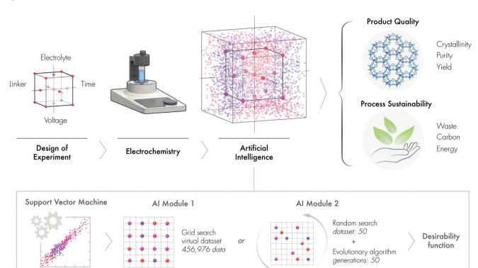
Fig. 1 Strategy for AI-based sustainable materials development in a hyperdimensional system. (a) General steps and process parameters to evaluate product quality and process sustainability in electroorganic synthesis of ZIF-8. (b) Simplified flow chart of the applied AI modules and machine learning.
