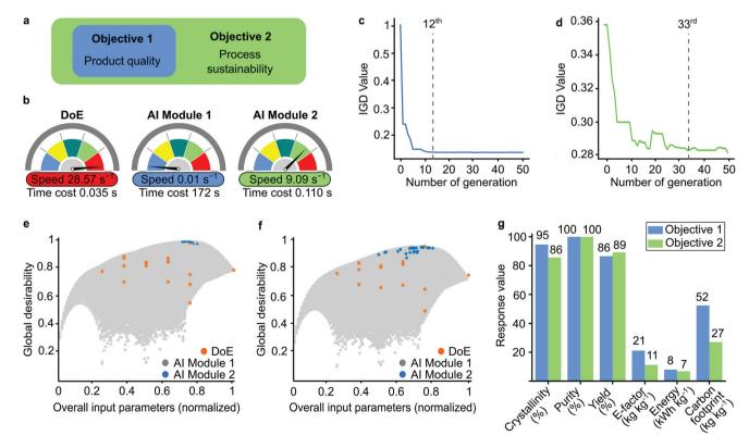
Fig. 4 Hyperdimensional optimization strategy. Expanding objectives for optimizations (a). Time cost for the DoE and Al modules as part of the whole system (b). Inverted generational distance (IGD) test over the number of generations in genetic algorithm for objectives 1 (c) and 2 (d). Global desirability for the overall input parameters for objectives 1 (e) and 2 (f) using three methodologies: DoE, Al Modules 1 and 2. Response values for Al Module 2 (g).
