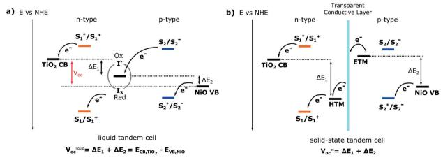
Fig. 5 Potential diagram of (a) the liquid based t-DSCs and (b) tandem solid state DSC where the liquid electrolyte is replaced by a solid-state hole transport material (HTM) for n-type cells and an electron transport material (ETM) for p-type cells.
