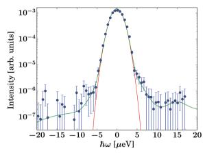
Fig. 2 Energy resolution function recorded at  $q = 1.08 \text{ Å}^{-1}$  using a vanadium standard in the same geometry as the samples (symbols), and fit (green line), being well described by a Gaussian over 3 orders of magnitude (red line)
