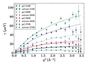
Fig. 7 Lorentzian width  $\gamma(q)$  associated with the PCM guest molecule (egn (2), symbols). The solid lines represent fits of the jump diffusion model (egn (3)).
