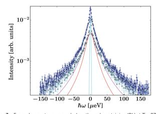
Fig. 3 Example spectrum recorded on the gel containing IBU at T = 270 Kand  $q = 1.08 \text{ Å}^{-1}$  (dark blue circle symbols). The light blue/black squares represent the corresponding pure solvent spectrum. The dark blue line superimposed on the circle symbols denotes the fit consisting of the guest molecule, solvent, and container contributions (egn (2))
