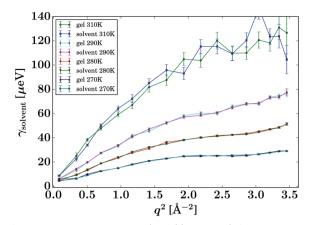
Fig. 4 Lorentzian widths  $\gamma_{solvent}$  (eqn (1), symbols) fitted to the pure solvent and pure gel spectra, respectively, for the samples and temperatures as given in the legend. The lines are guides to the eye.
