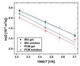
Fig. 9 Summary of the jump diffusion coefficients D (eqn (3), symbols) associated with the guest molecule diffusion in an Arrhenius plot for all samples as given in the legend. The lines report linear fits to obtain the Arrhenius activation energies (eqn (4)).
