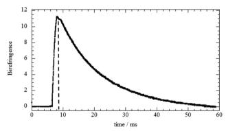
Fig. 4 Transient electric-field-induced birefringence signal for aqueous dispersion with a HPC/HNT mass ratio of 0.1. The HNT concentration was 0.15 g dm<sup>-3</sup>. The experiments were conducted using rectangular pulses (the applied electric field and the pulse length were fixed at  $1.25 \times 10^5 \, \mathrm{V m}^{-1}$ and 2.5 ms, respectively). The dashed line represents the time point where the electric field was switched off.
