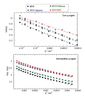
Fig. 2 Guinier plots for HNT/chitosan, HNT/alginate, HNT/HPC and HNT dispersions in D<sub>2</sub>O within the low (0.007 nm<sup>-1</sup>  $\leq q \leq$  0.009 nm<sup>-1</sup>) and the intermediate (0.015  $\text{nm}^{-1} \le q \le 0.02 \text{ nm}^{-1}$ ) regions. The low q Guinier plot is ln(I(q)) vs.  $q^2$  (top), while the intermediate q Guinier plot is  $ln(q \cdot I(q))$ vs.  $q^2$  (bottom). Dashed lines represent the fitting according to eqn (1) and (3).
