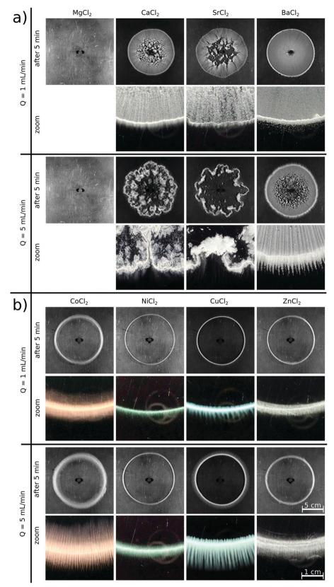
Fig. 1 Grayscale images of the precipitation patterns observed in the different chemical systems with direct injection for various flow rates 5 minutes after the end of the injection ( $V_{\text{max}} = 5 \text{ mL}$ ). Close-ups of the macroscopic patterns shown in real color.
