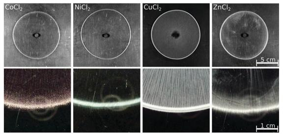
Fig. 3 Grayscale images of the precipitation patterns observed in the different chemical systems with reverse injection at Q = 1 mL min<sup>-1</sup> flow rate 5 minutes after the end of the injection ( $V_{\text{max}}$  = 5 mL). Close-ups of the macroscopic patterns shown in real color
